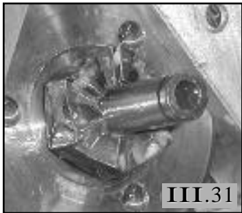
III.31 Inspect both sides of clutch nut assembly for wear or breakage, replace as needed.
