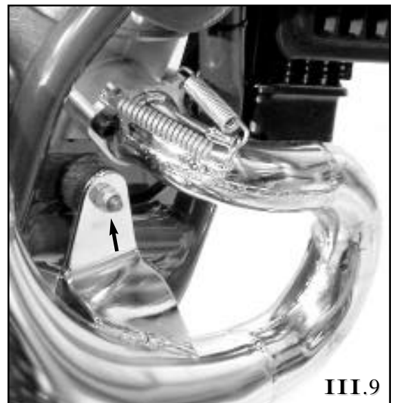
Remove 2 springs, and nut from exhaust mount.
