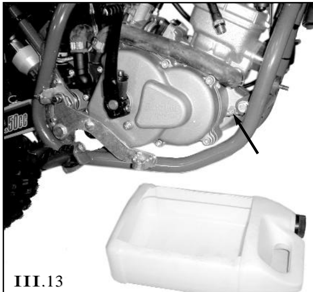
III.13 Remove radiator cap & drain coolant using bleed screw
