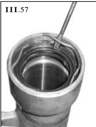
Use screwdriver to remove seal retaining ring.
