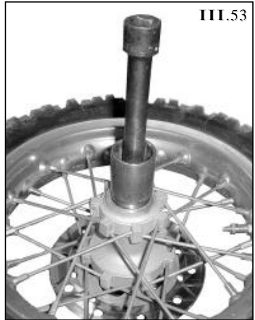
Use large socket to drive bearing in squarely.
