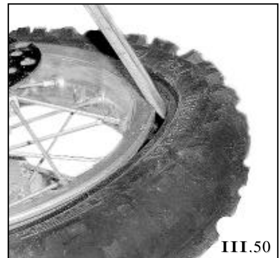
Do not pull tire iron too far to reduce chance of pinching tube
