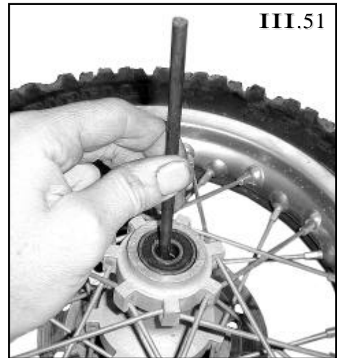
Use rod at angle to drive out opposite wheel bearing.
