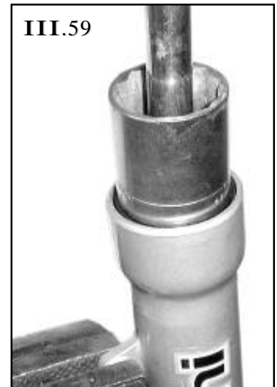
Installing oil seal into fork slider.
