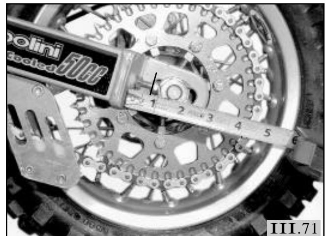
Make sure axle is same distance on each side.
