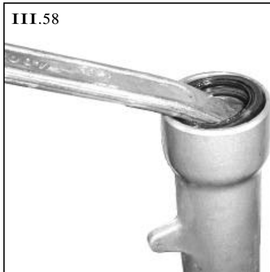
Use blunt tool to remove inner seal.
