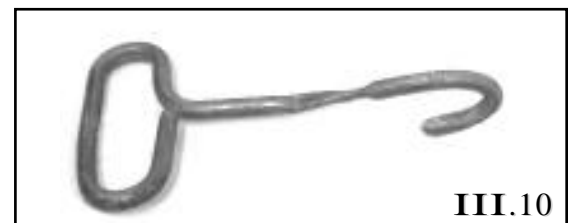
Homemade spring removal tool.
